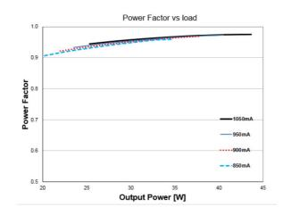
OT FIT 40 CS T Typical Power Factor vs. Load
